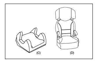
A booster seat (C-D) is a child restraint designed to improve the fit of the vehicle's safety belt system. A booster seat can also help a child to see out the window. Securing an Add-On Child Restraint in the Vehicle
